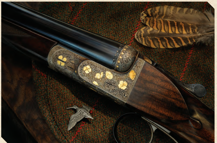
Working from chopper-lump barrel forgings, the guns of Jagdwaffen Ern are made entirely in the family's shop by a mix of traditional craft methods and modern, computer-controlled machinery. Evelyn's engraving (below) is "much inspired by nature."
